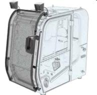
Cabin guard at front for protection against damage.
