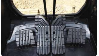
Rubber coated track pedal and foot rests for operator comfort. Front lower glass can be removed for ventilation.
