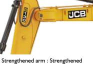
boom joint and bucket joint area. Additional plate provided at bottom for damage protection.
