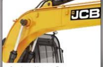
Reinforced boom : Deep section design, reinforced base area and cylinder mounting area for higher
