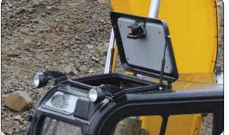
Roof hatch provided to keep the cab well ventilated, which is aided by rear sliding window. Additional cab top lights for better illumination.
