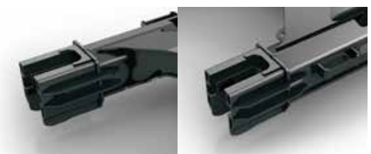
Heavy duty track frame with idler area reinforcements
