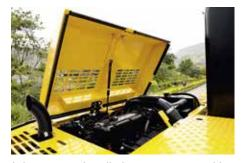
Compact and the easy-to-handle bonnet is assisted by a gas strut that helps in easy opening and closing. It makes periodic maintenance easy and effortless.
