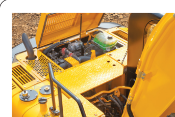
Compact size engine bonnet helps in easy and effortless handling during the maintenance.
