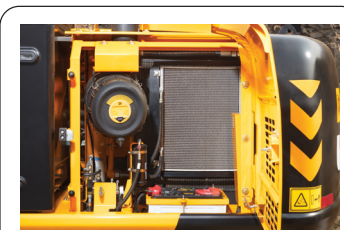
Wire mesh guard on the cooling pack to prevent entry of debris or other objects.
