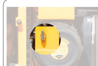
Battery disconnect switch helps to isolate the machine's electric system easily, whenever required.
