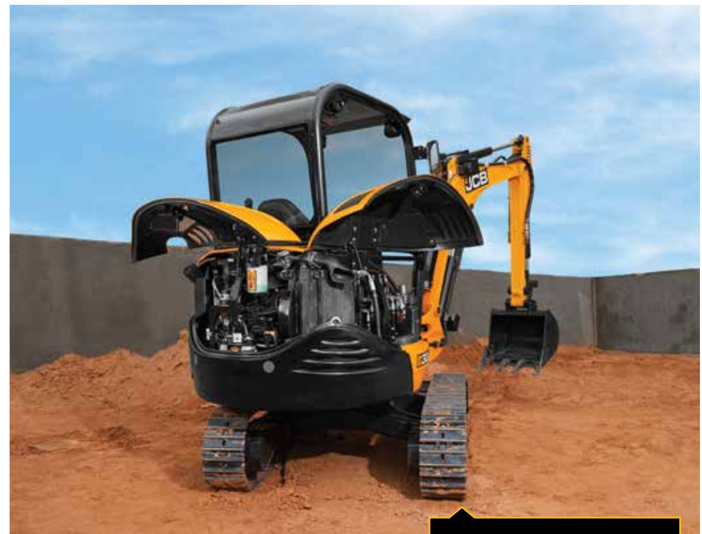
Wide-opening service access panels are supported by gas struts for excellent access to routine checks.
