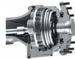
3 Hydraulic power, oil immersed Brakes
